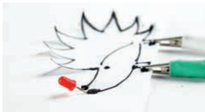
Draw a simple shape with conductive ink to complete the circuit, and it completes an action, for example, light an LED.
