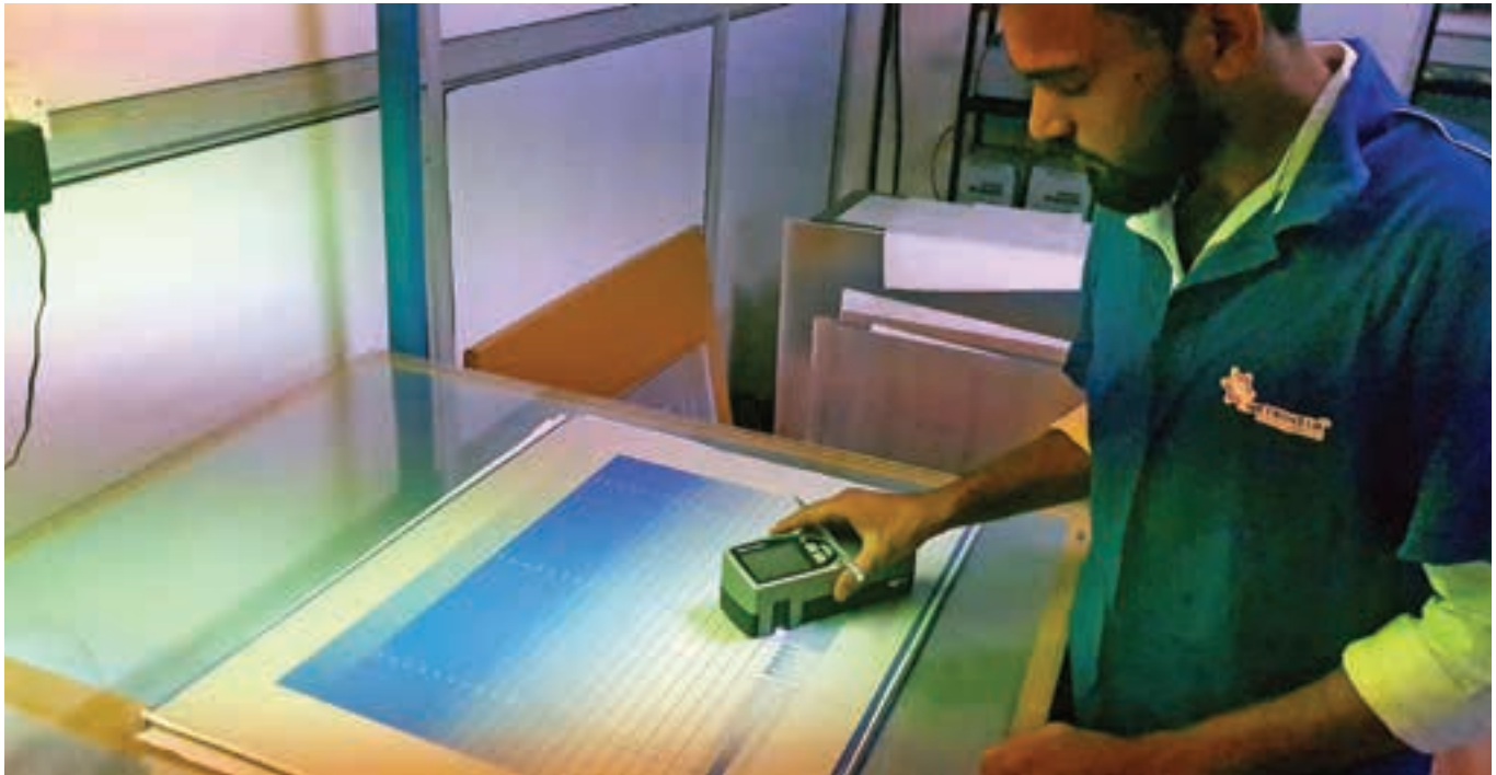
The final product is checked for weight and the consistency of the coating, RA values, graining structure through a 400x microscope camera, and expose a plate to check all the parameters, including, 1%, 3%, 50% dot.
