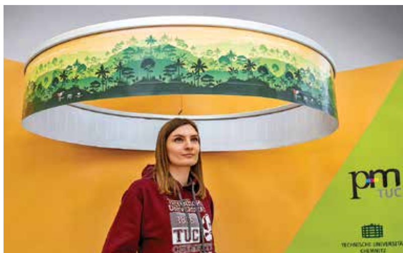
Printed speakers create a surprising jungle illusion. Printed electronics embedded in a paper web enable 360° surround sound. Varvara Bachul from the Institute of Print and Media Technology at the Chemnitz University of Technology analyses the sound generated inside the T-RING. The sounds come from 56 individually printed loudspeakers that are connected to form seven segments on the circular track, which is almost four meters long. Photo: Jacob Müller.
