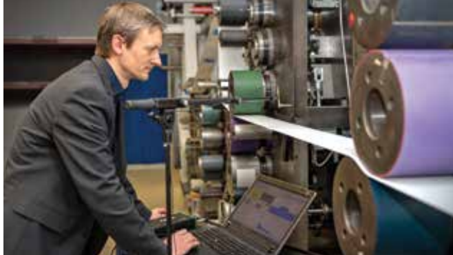
A novelty of the Chemnitz innovation is the acoustic inline characterisation. Project manager Dr Georg C. Schmidt acoustically tests the completely printed paper loudspeaker web on a roll-to-roll printing machine and can thus assess its quality. Photo: Jacob Müller
